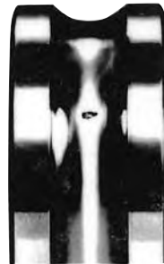
Fig. 5.1 Example of Flaking
